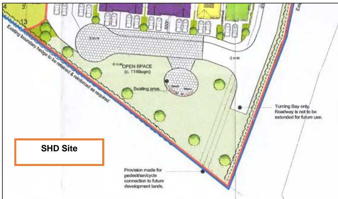
Figure 10: Extract from site layout plan of Reg. Ref.: RA160065, showing future cycle / pedestrian linkage
